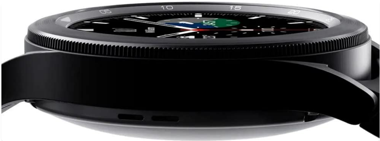
Figure 2: Side view of the Samsung Galaxy Watch 4 Classic, showing the rotating bezel and side buttons for navigation.
