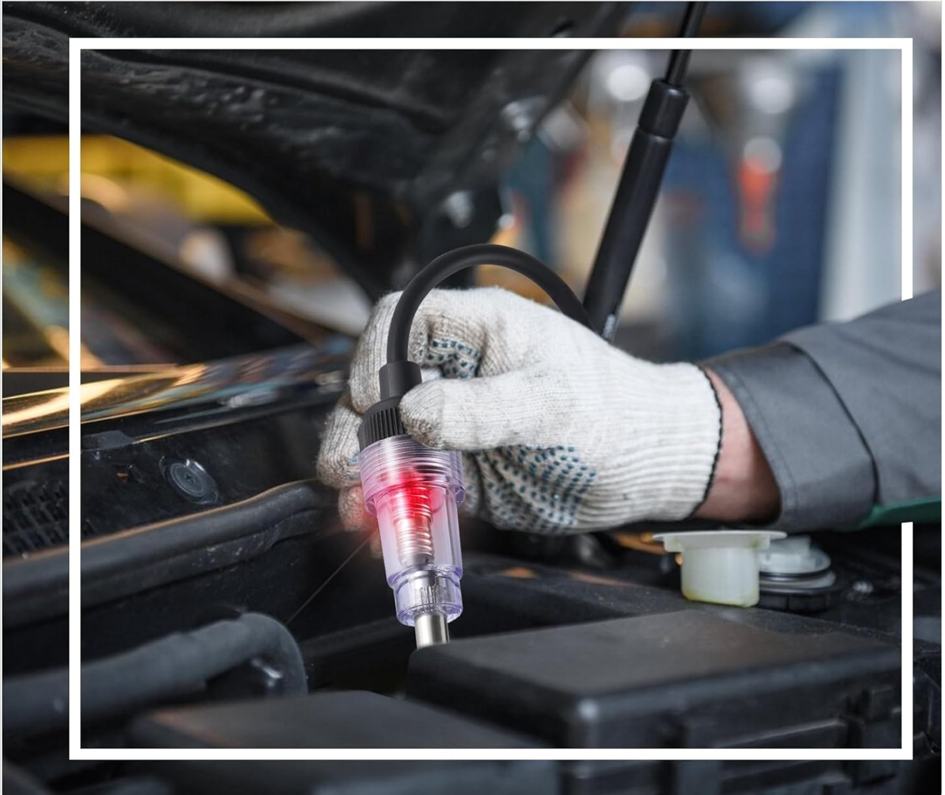
Figure 6: The tester in operation, with the internal bulb illuminating to indicate spark.
