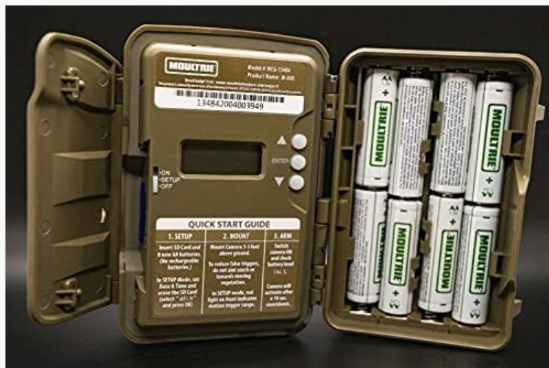
Image: An open Moultrie W800 camera, revealing the battery compartment on the right, the control panel with a small screen, and buttons on the left. This view is essential for battery and SD card installation.
