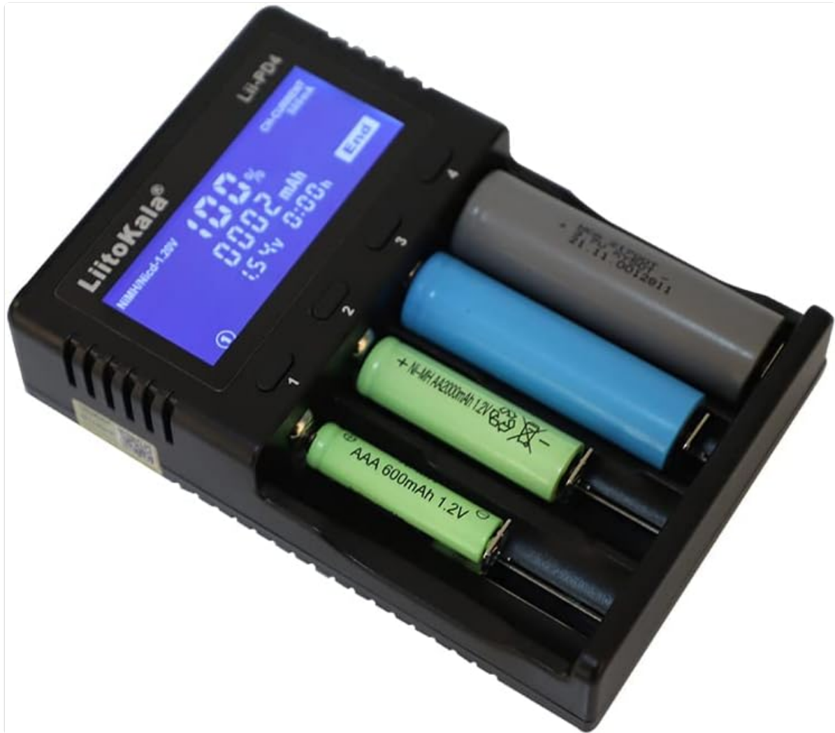
Figure 3: The charger with different types of batteries inserted into its four independent bays.
