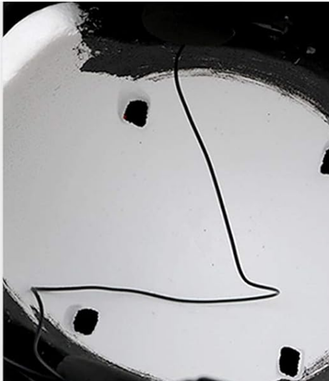
Figure 5: Visual guide for speaker and microphone placement within the helmet.
