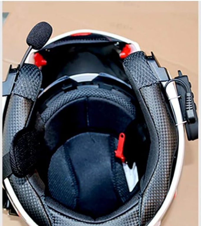
Figure 5: Visual guide for speaker and microphone placement within the helmet.
