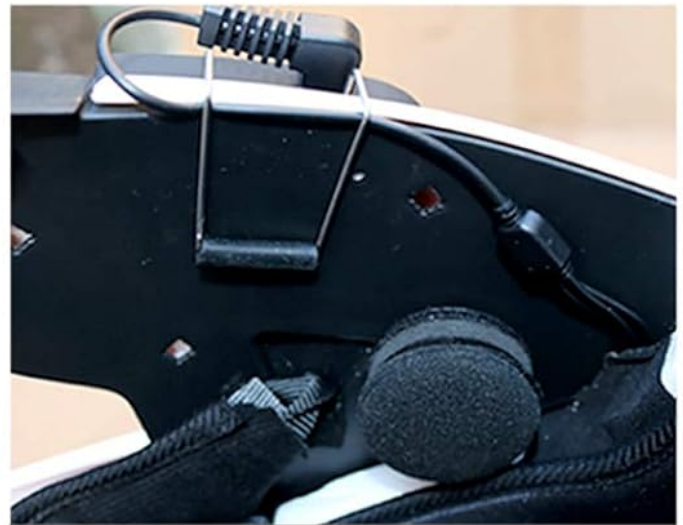
2. THE HOST IS USUALLY INSTALLED IN THE LEFT HAND, AND THE MICROPHONE IS USUALLY IN THE RIGHT HAND.
