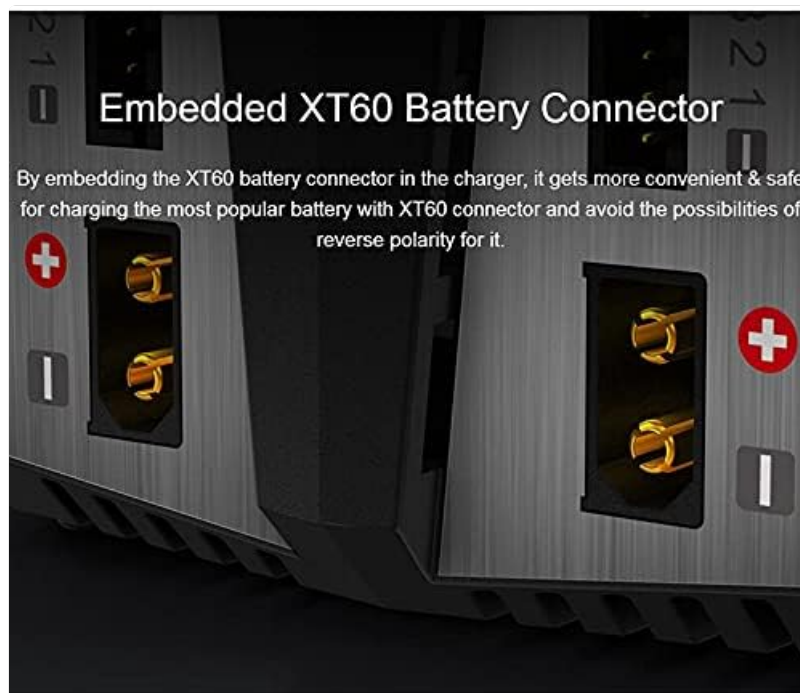
Image 3.6: Close-up view of the embedded XT60 battery connectors on the SKYRC T100 charger, designed for secure and convenient battery connection.
