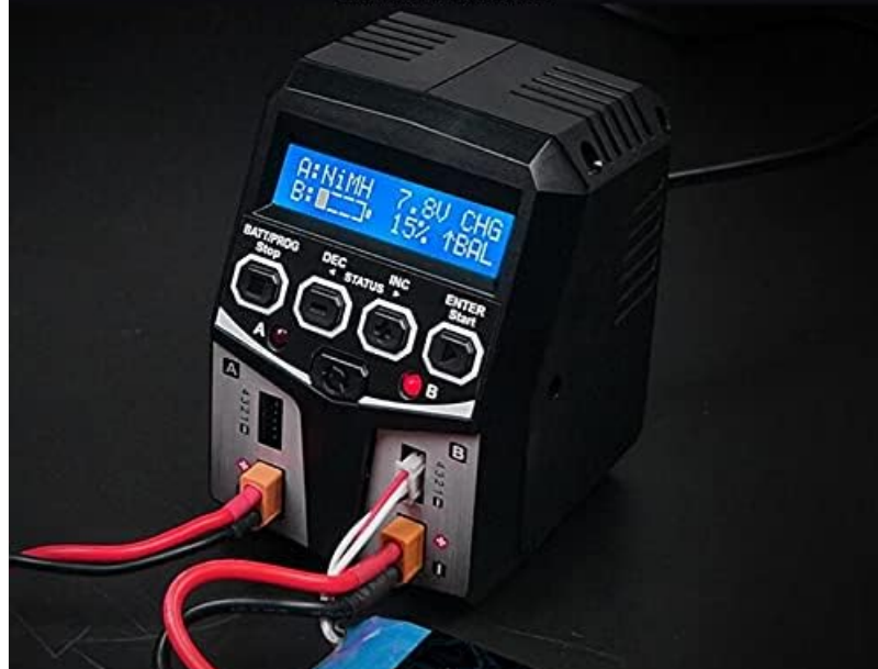
Image 3.3: The SKYRC T100 charger with two batteries connected, demonstrating its twin-channel charging feature. The display shows charging status for both channels A and B.
