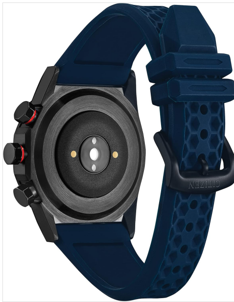
Back view of the Citizen CZ Smart Hybrid Smartwatch, highlighting the heart rate sensor and charging contacts.
