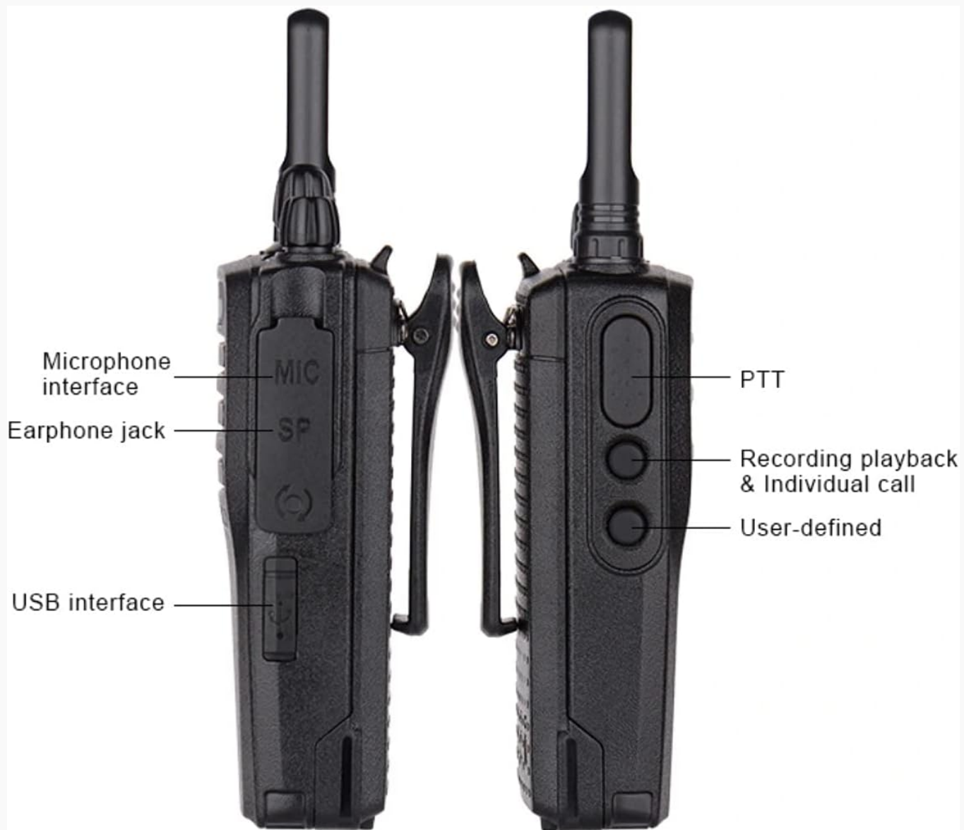
Figure 2.2: Side View of T529A Radio with Labeled Interfaces and Buttons.
