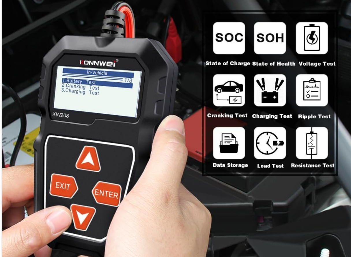
Image: The KW208 screen showing icons for different test modes: State of Charge, State of Health, Voltage Test, Cranking Test, Charging Test, Ripple Test, Data Storage, Load Test, and Resistance Test.
