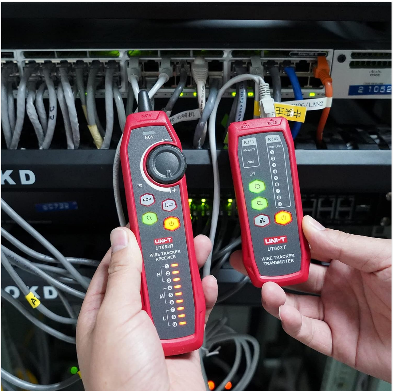
Image 5.1: The UT683KIT being used to trace cables connected to a network switch.
