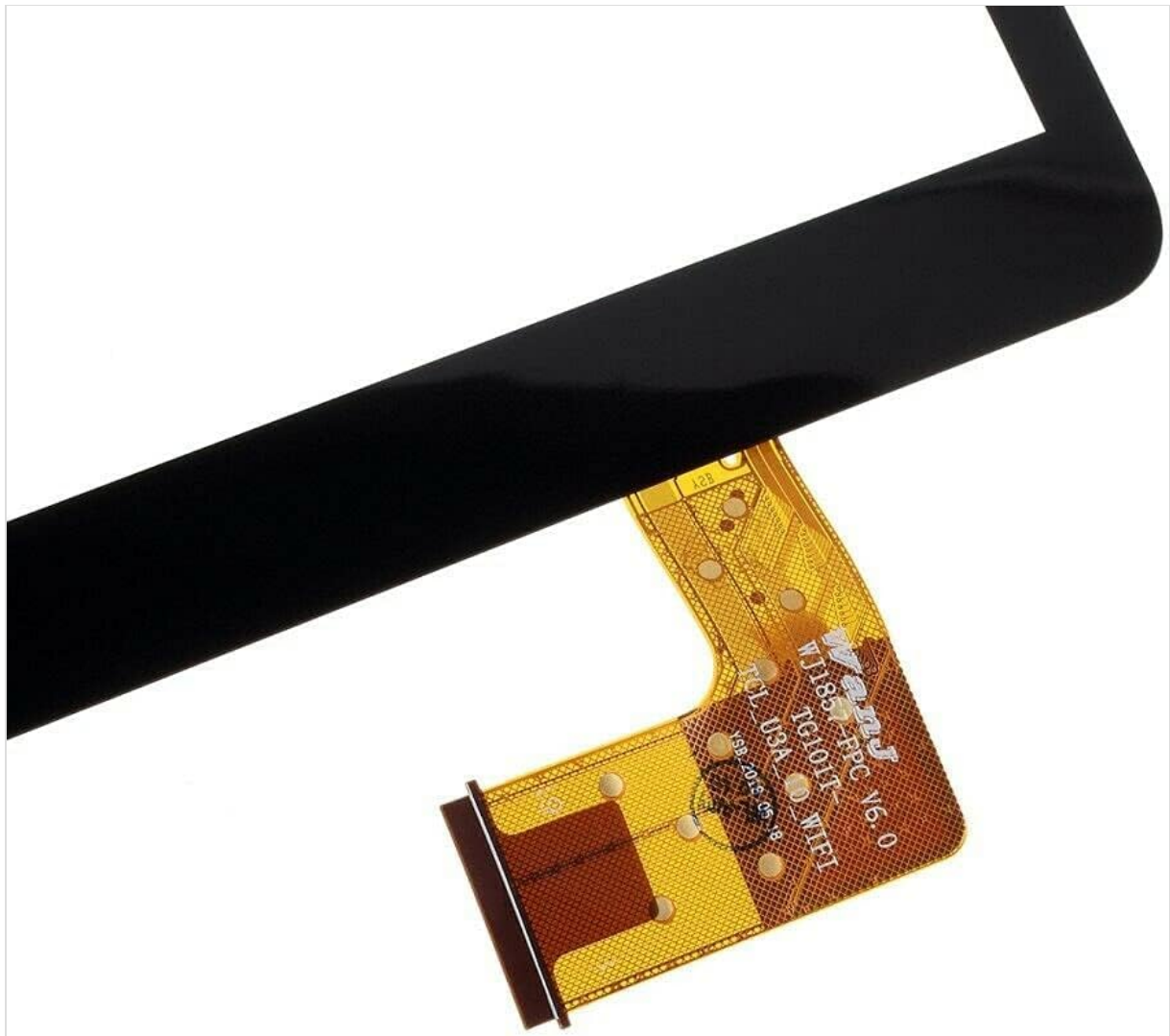
Image 4: Detailed close-up of the flex cable and connector, essential for tablet integration.
