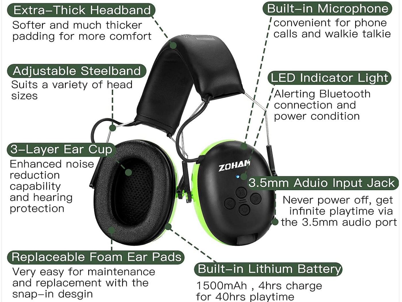
Image: Detailed breakdown of ZOHAN EM037 components and features.
