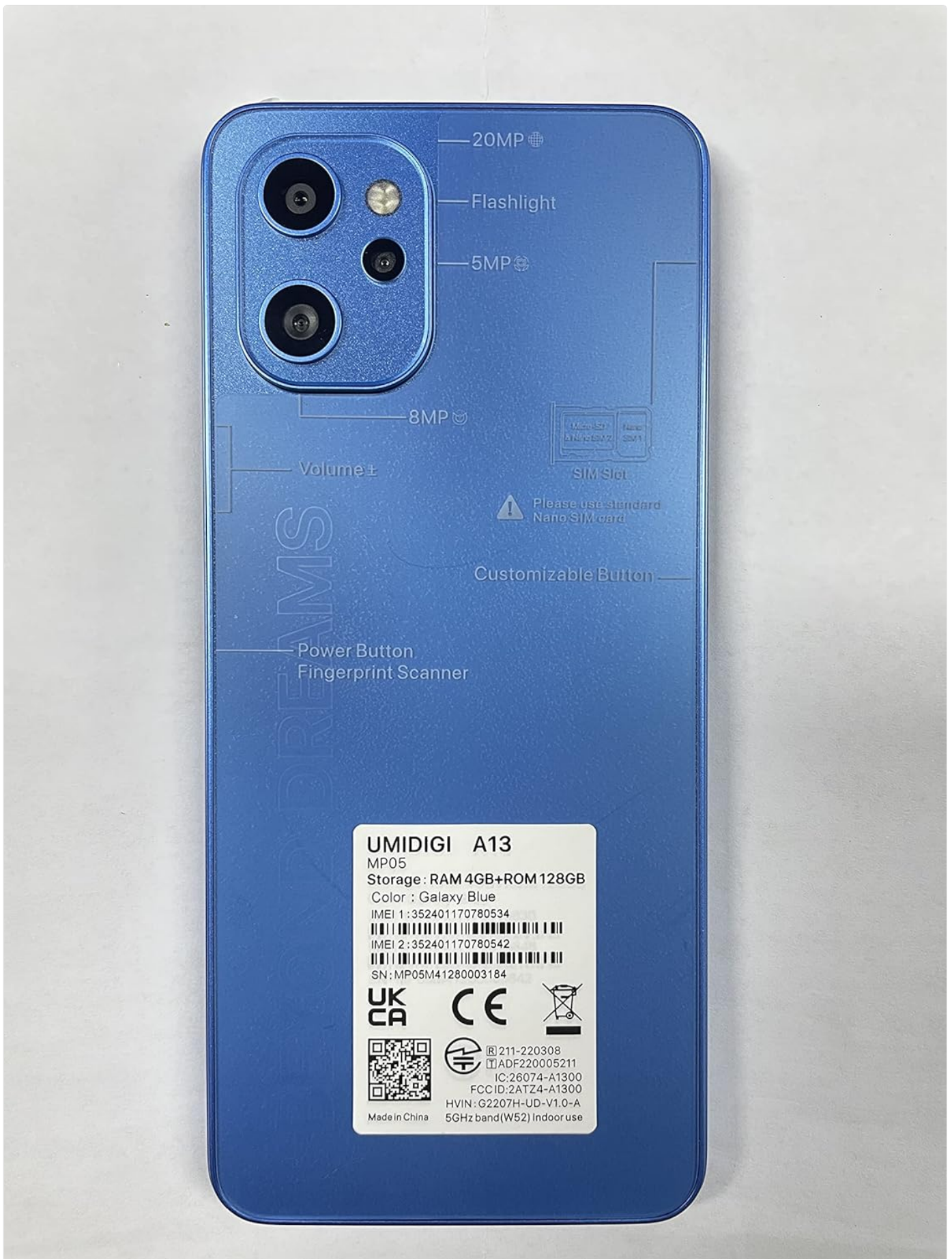
Image: The back of the phone with labels pointing to the volume buttons, power button/fingerprint scanner, customizable button, and SIM slot.
