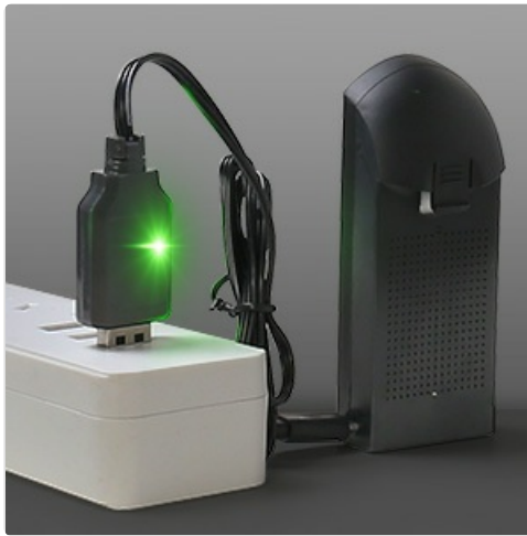
Image: Proper method for charging the drone battery using the provided USB cable.
