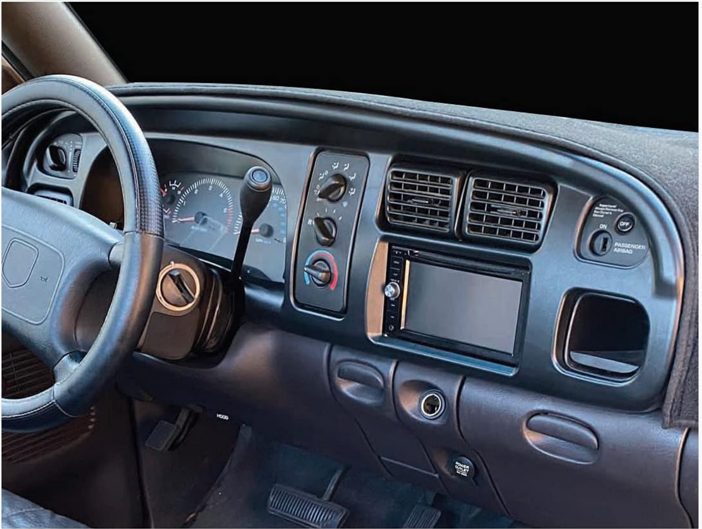
Figure 4: Example of the Metra DP6551 dash kit installed in a vehicle with an aftermarket Double-DIN radio.
