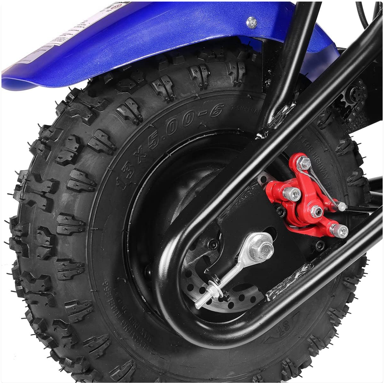
Image 2: Detail of the rear disc brake system.
