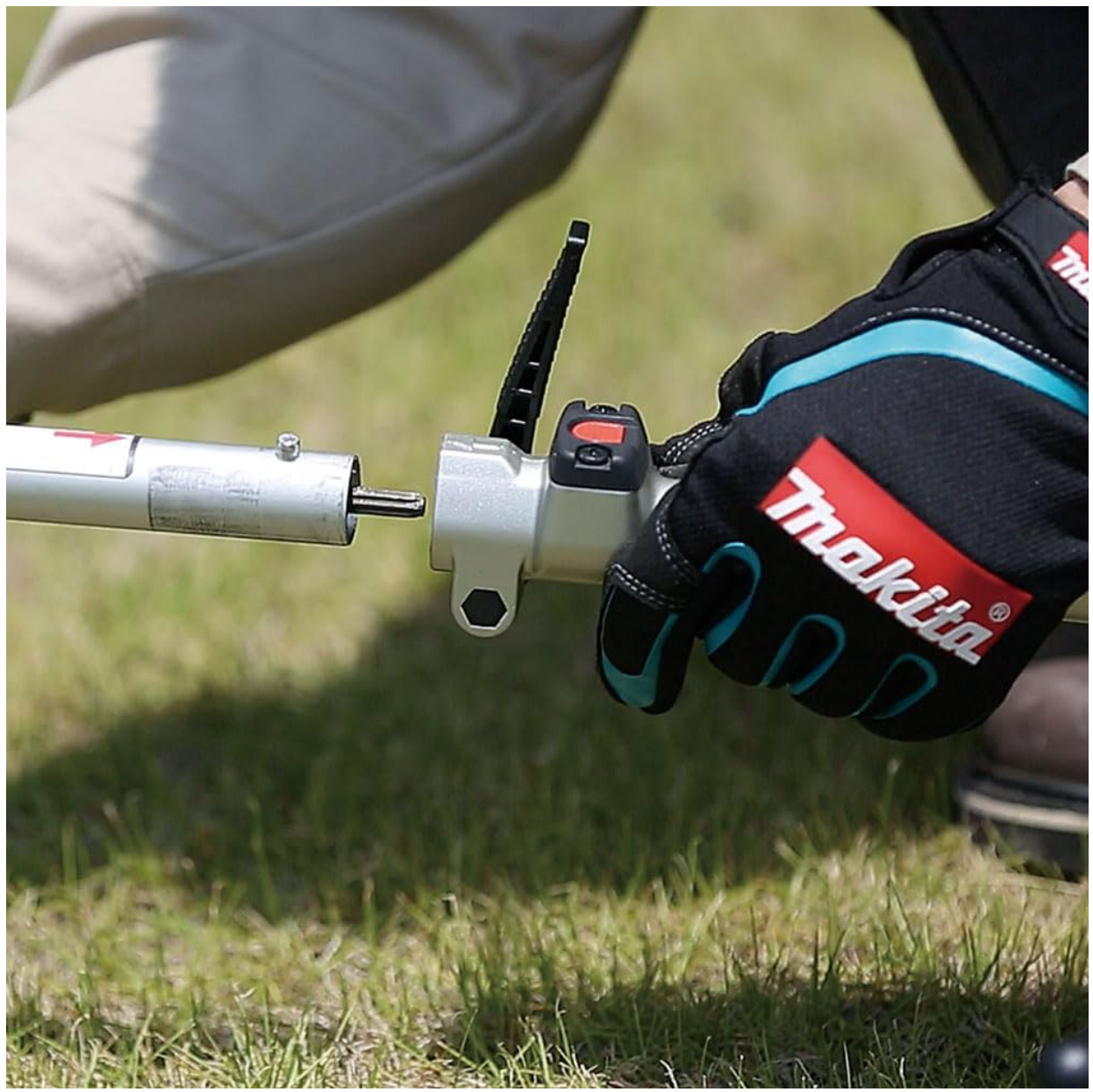
Figure 2: A close-up view demonstrating the process of attaching the blower shaft to the power head, highlighting the alignment of the pin and coupling.
