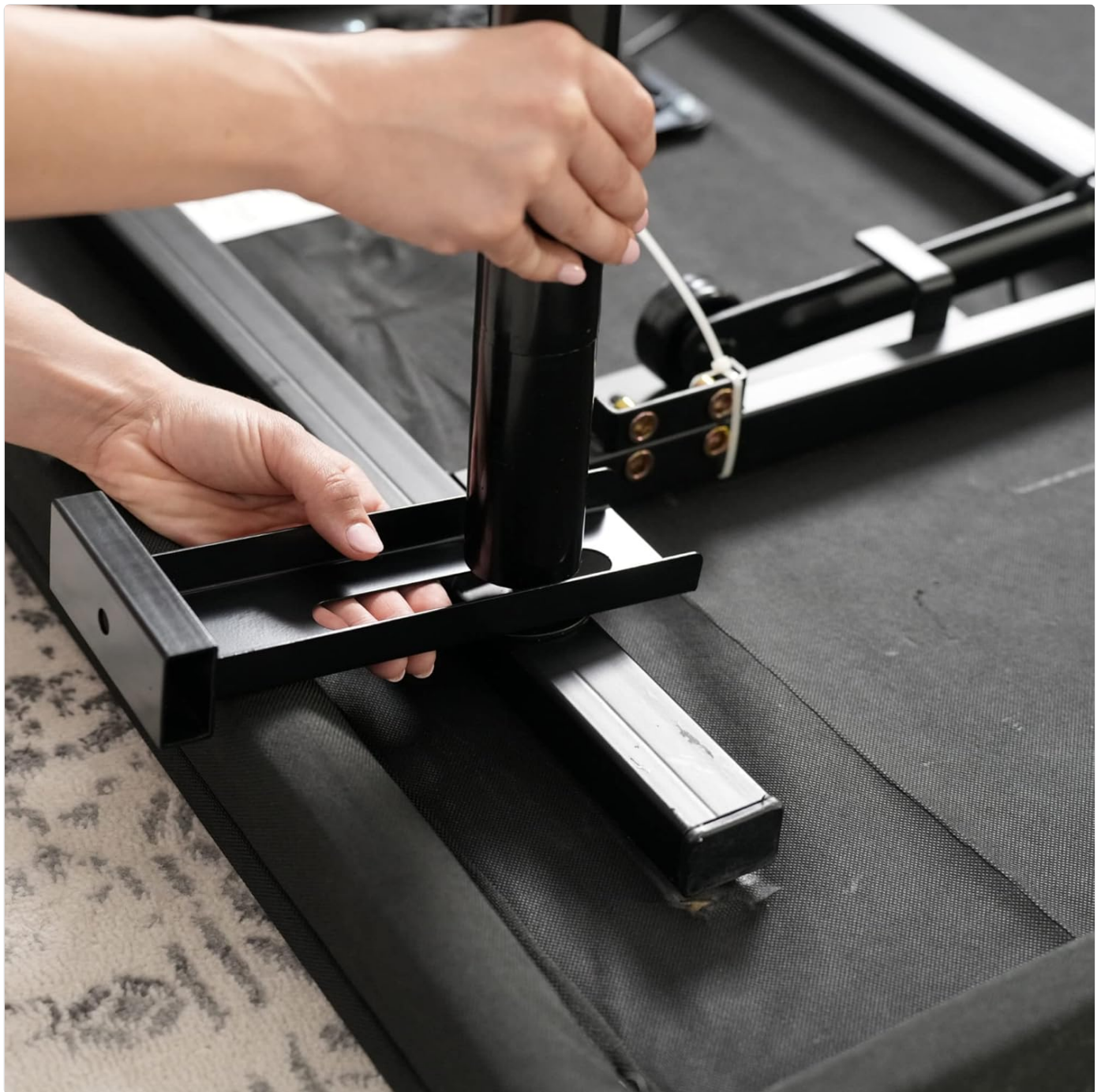
Figure 2: Attaching the T-shaped bracket to the adjustable bed frame.
