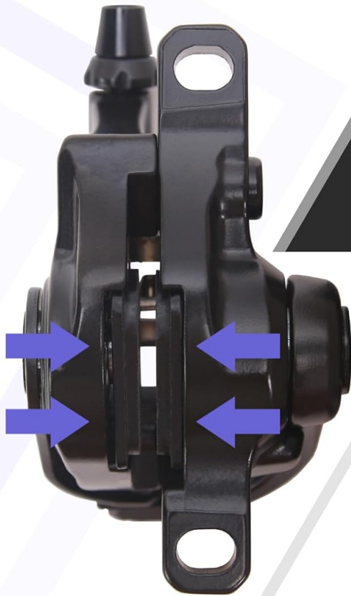
Figure 2.3: Illustration comparing the double piston drive work with a unilateral drive friction plate. The double piston system applies even stress to the brake rotor, preventing deformation and ensuring stable braking. A unilateral system can cause rotor deformation, uneven friction, and limited braking force.
