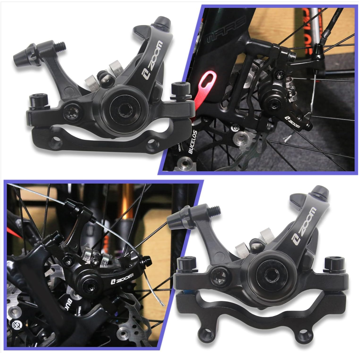
Figure 3.2: Examples of the BUCKLOS mechanical disc brake calipers installed on a bicycle, demonstrating proper mounting and cable routing.
