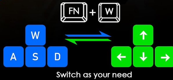
Image: Illustration of the FN key combination to switch W/A/S/D keys to arrow key functionality.
