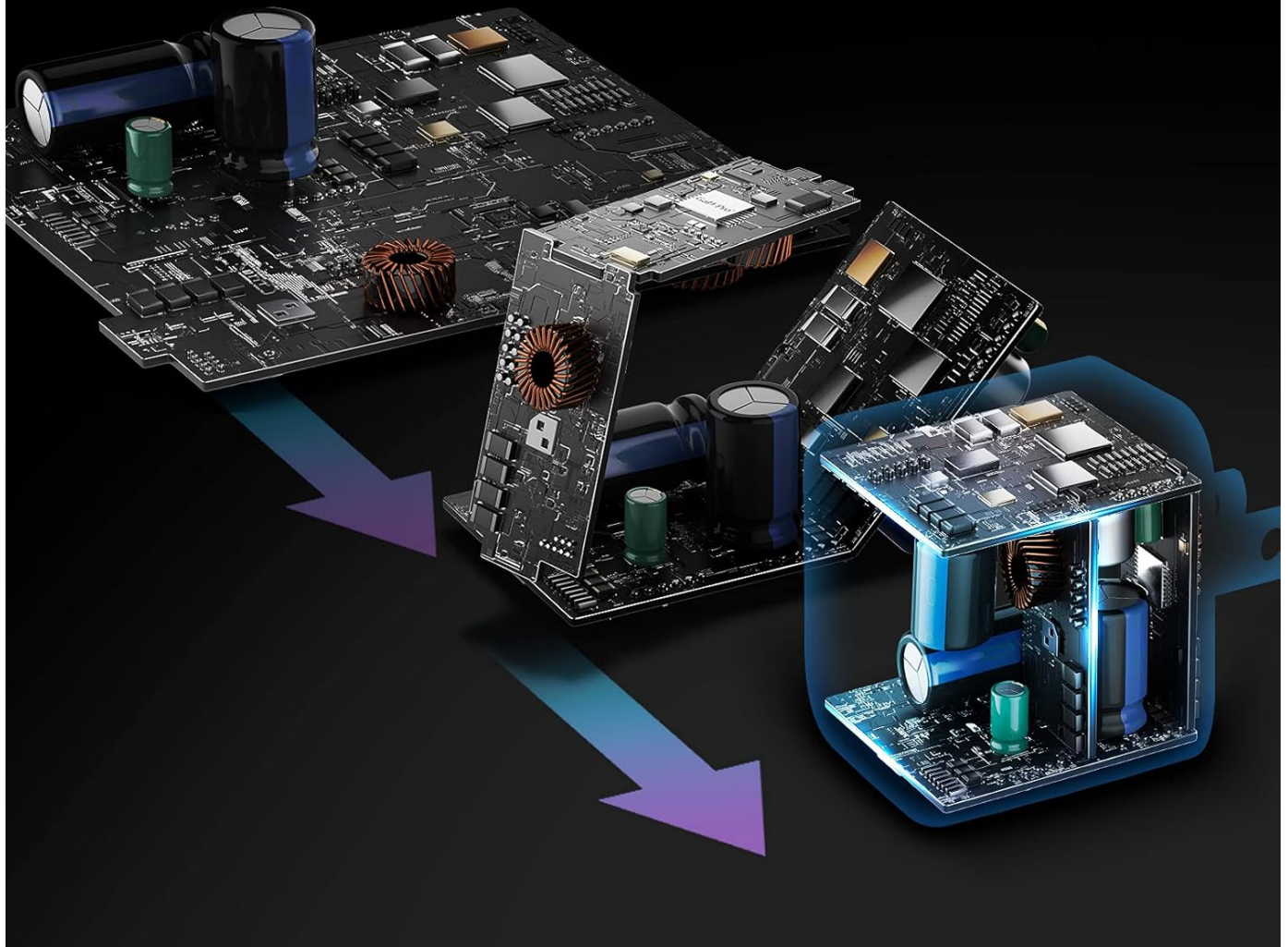
Figure 5: Internal 3D PCB Technology enables a smaller form factor.
