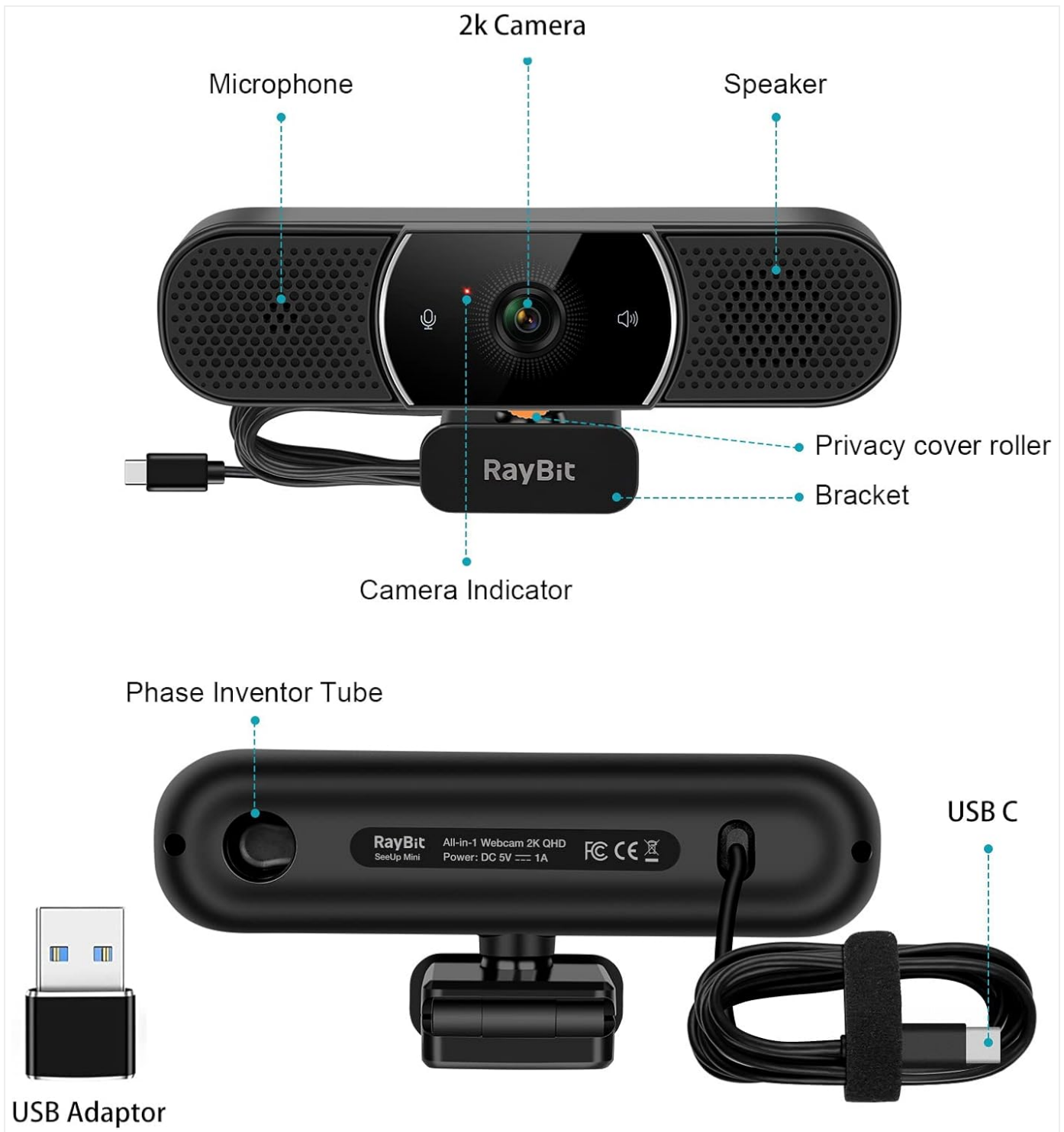
Image 1.4: Detailed component diagram of the SeeUpMini webcam, highlighting its integrated features.
