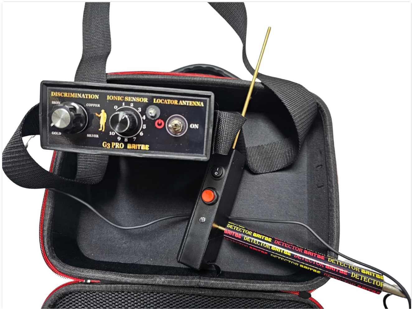
Figure 3: The G3 Pro control unit with the locator antenna properly connected.
