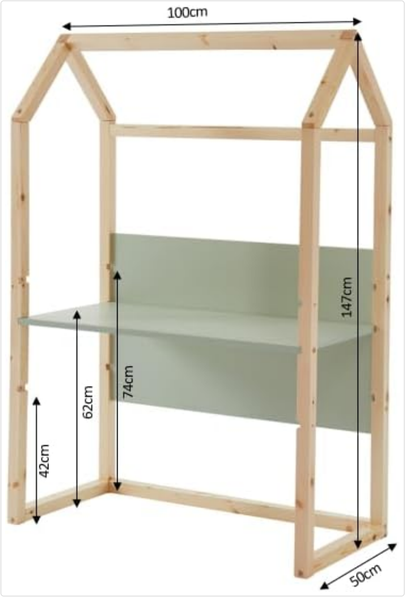
Figure 4: Dimensional diagram of the BAĬTA Children's Hut Desk.
