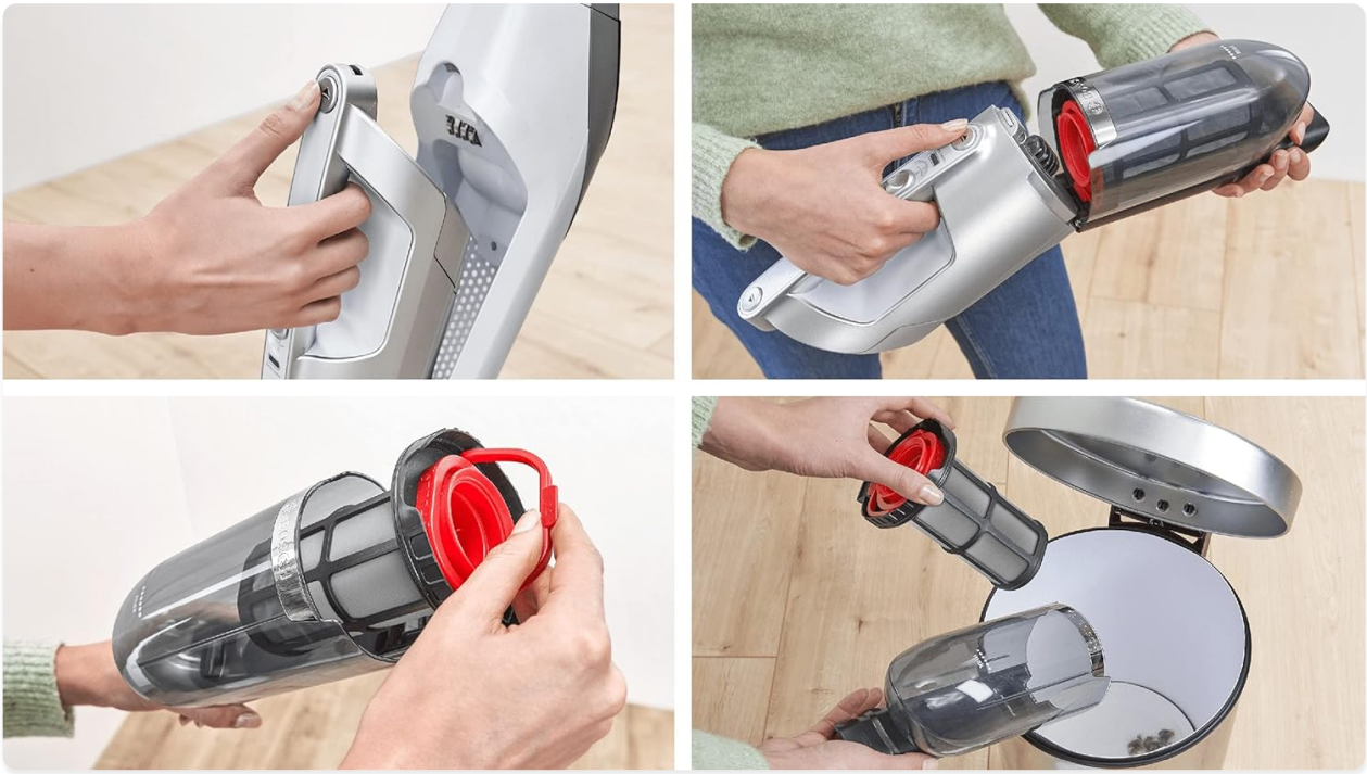
Figure 5.1: A four-panel image illustrating the process of detaching the dust container, removing the filter, and emptying the contents into a bin.
