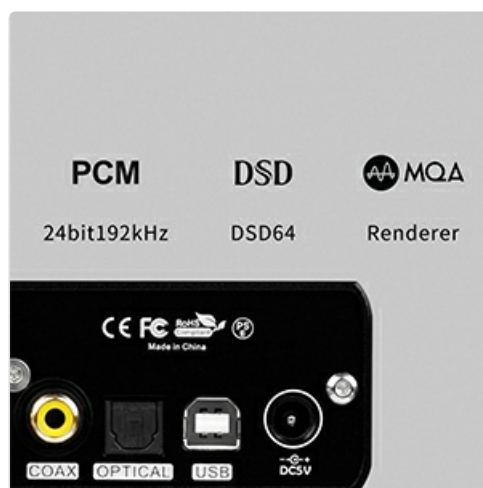
Image: Rear panel of the Topping E50, showing USB, Optical, and Coaxial input ports, along with power input.
