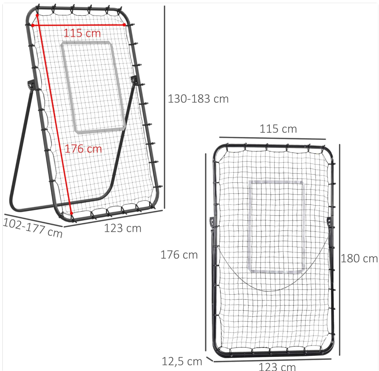
Image: Dimensional diagram of the rebound net, illustrating its various measurements and foldable design.
