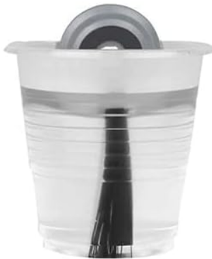
Figure 5: A visual guide demonstrating the four steps to straighten bent side brushes: identifying a bent brush, soaking it in hot water, allowing it to soak for minutes, and then removing and shaking off excess water to dry.
