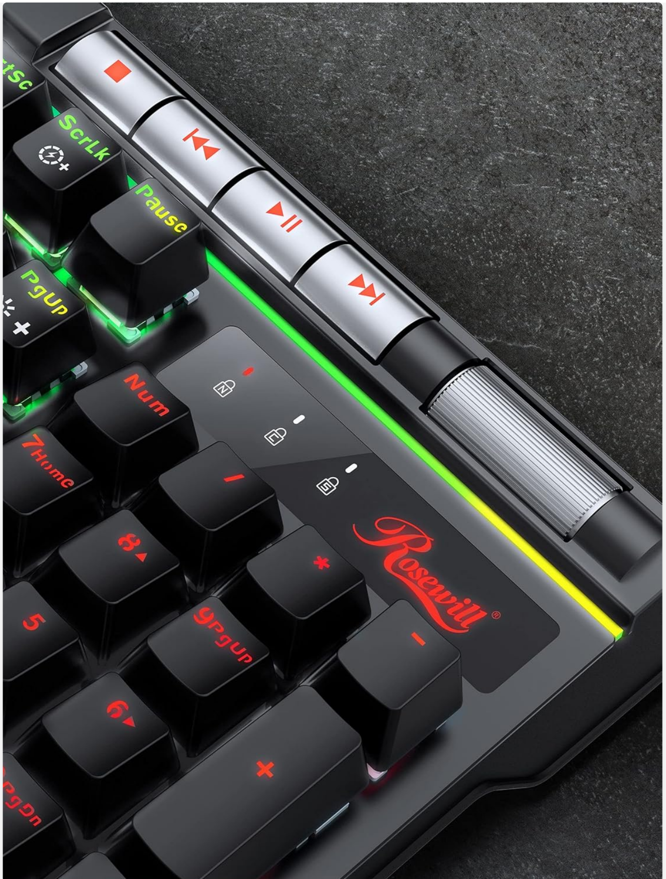
Image: A detailed view of the multimedia control buttons and the metallic volume roller located on the top right of the keyboard, highlighting their accessibility.
