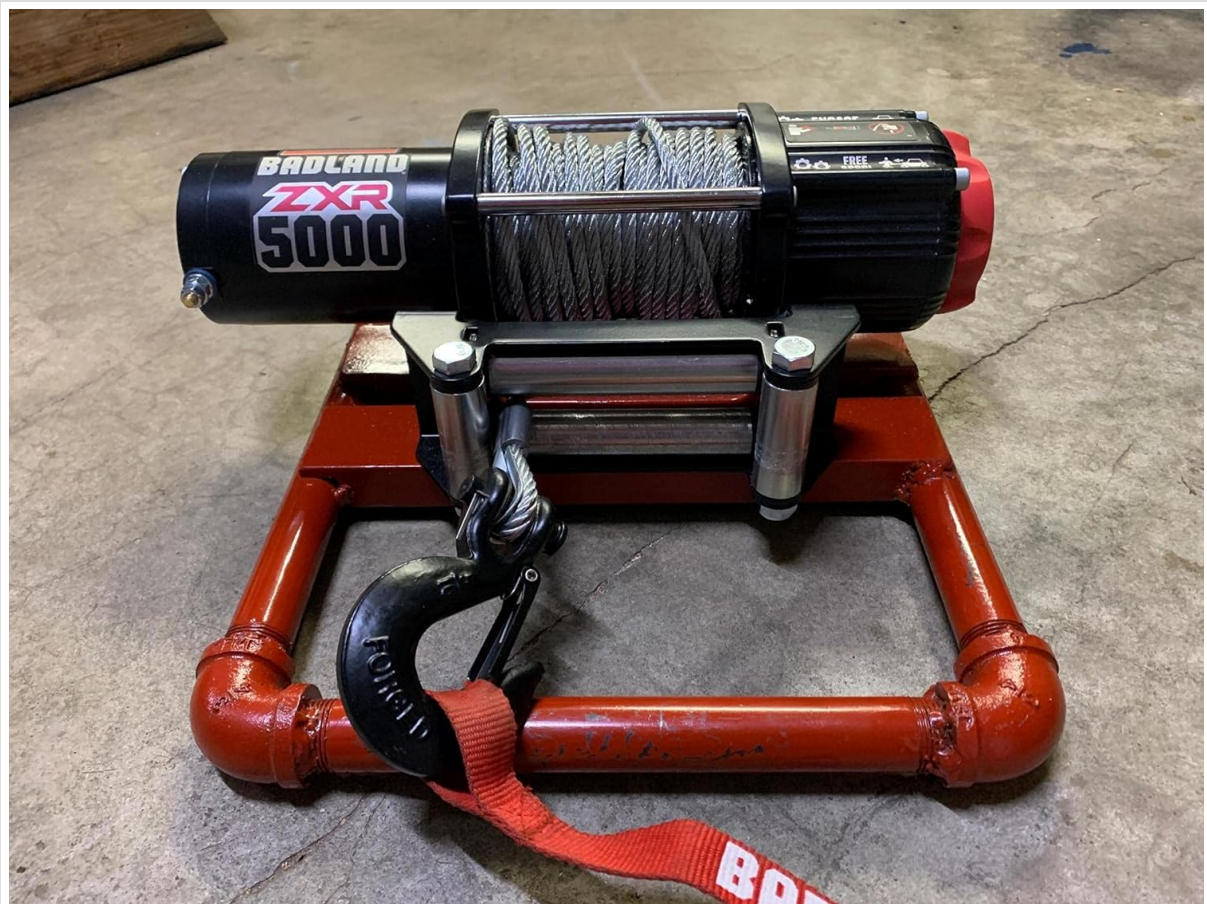
Figure 3: Detail view of the winch, highlighting the clutch lever (often labeled "Free Spool" or "Engage") and control markings.
