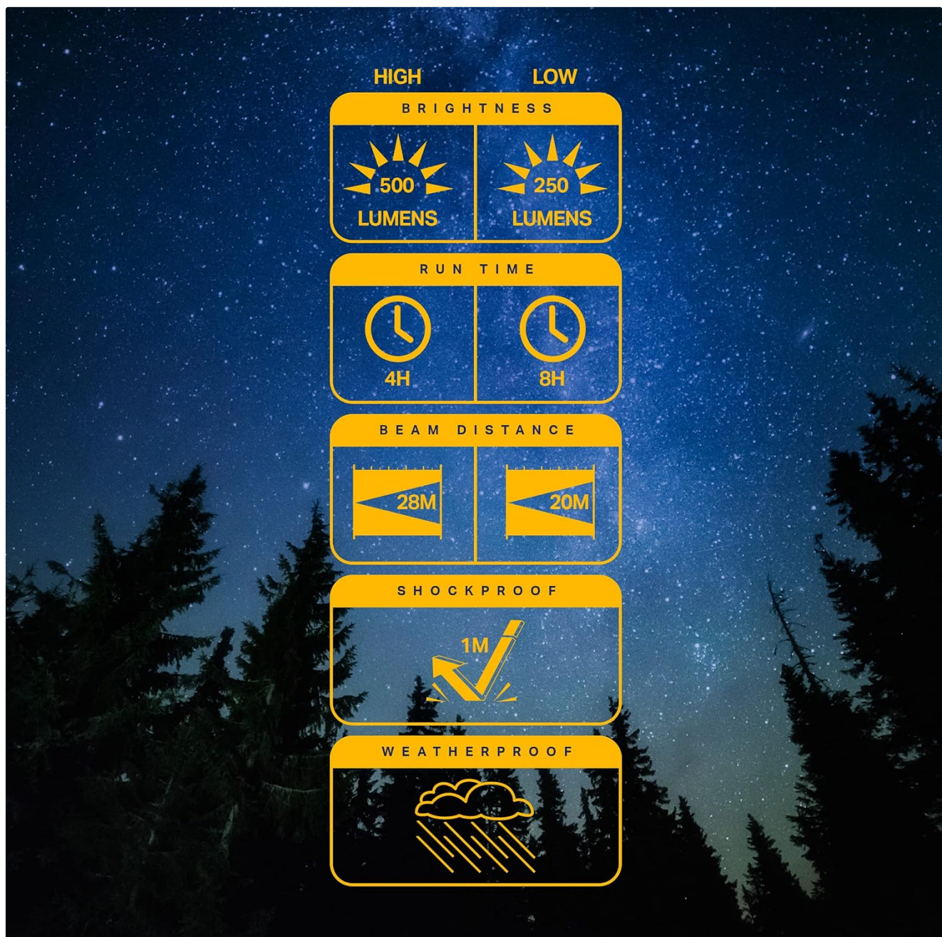
Figure 4: A graphic detailing the brightness, run time, beam distance, shockproof rating, and weatherproof rating of the LP385. It shows High brightness at 500 lumens for 4 hours and Low brightness at 250 lumens for 8 hours.
