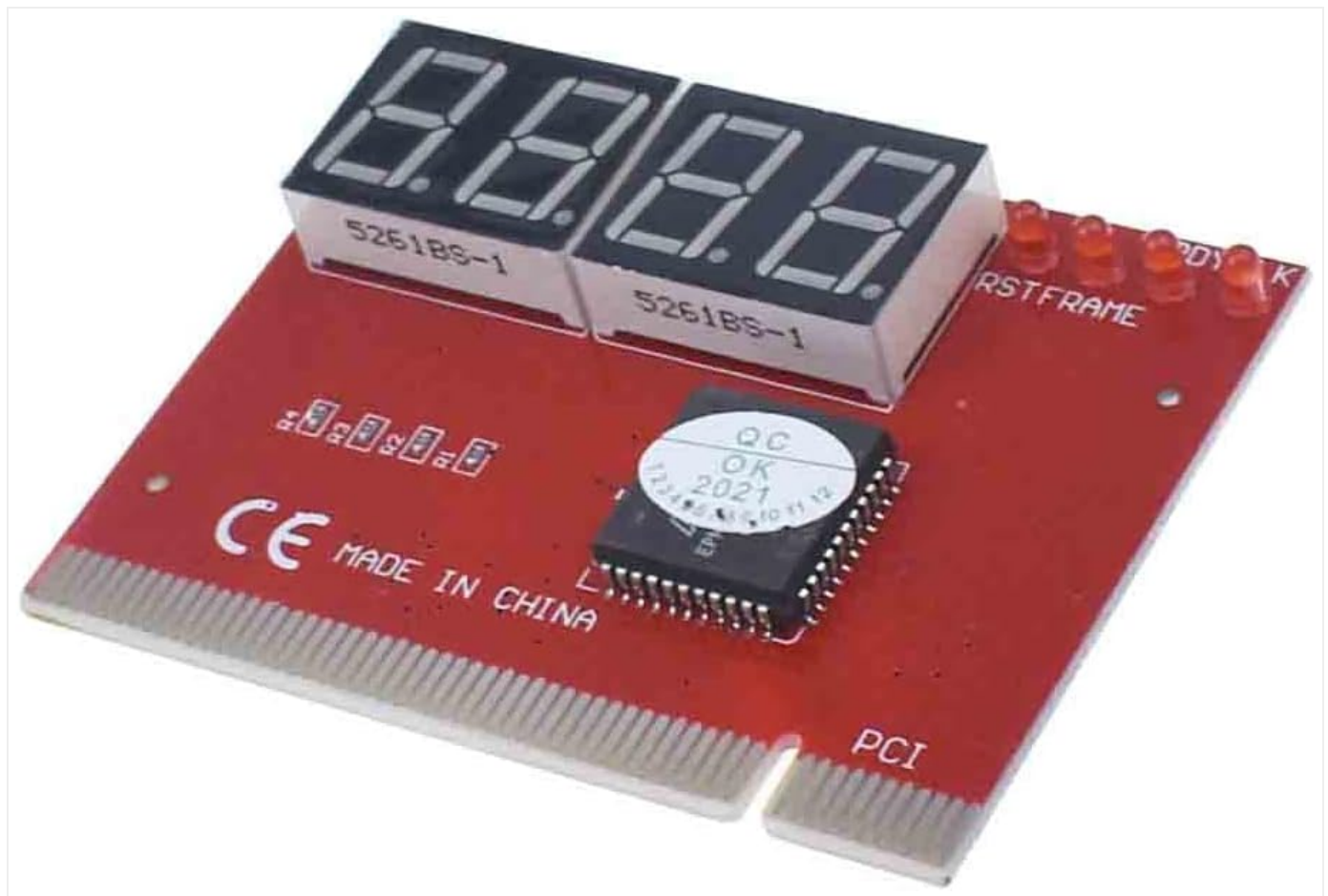
Figure 3: The diagnostic card ready for insertion into an expansion slot.
