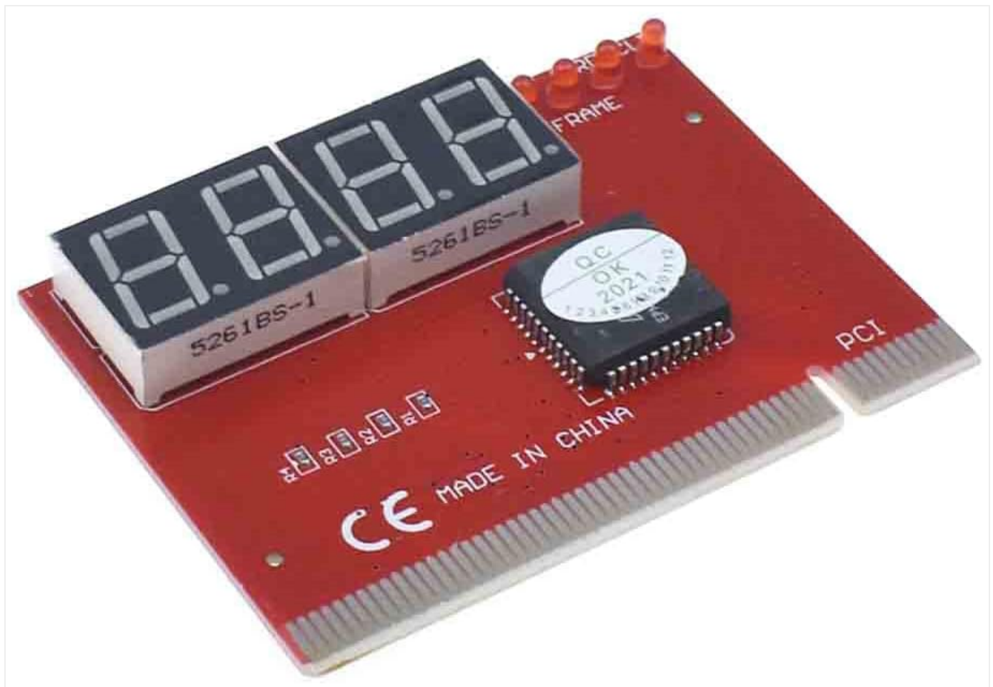
Figure 2: Detailed view of the diagnostic card, highlighting the 4-digit display and various onboard components.
