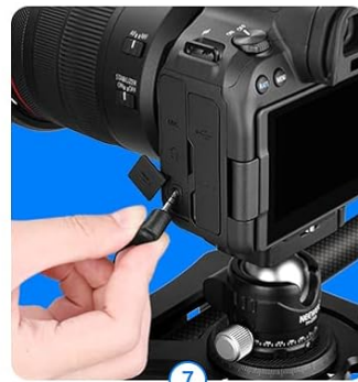
Insert the other end of the shutter release cable into the camera.
