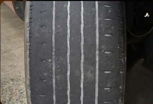
Uneven Tire Wear
