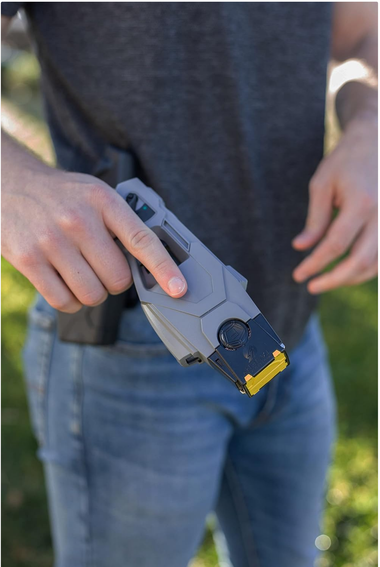
Figure 5.1: Proper insertion of a cartridge into the TASER X1 device.
