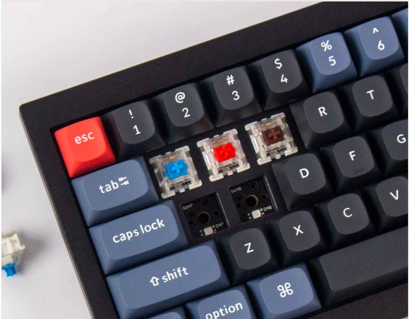
Image 4.3: A close-up view of the keyboard's PCB with several switches removed, demonstrating the hot-swappable feature.
