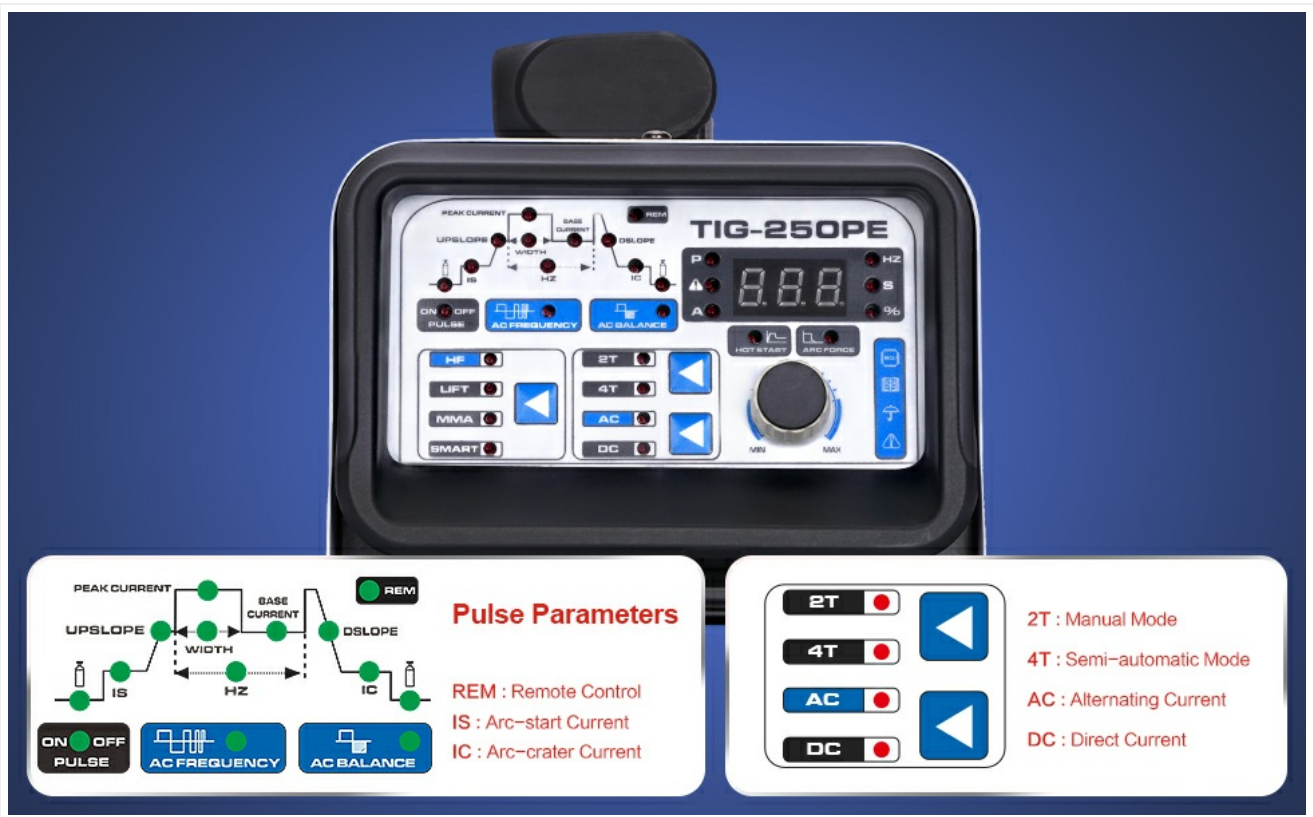
Figure 3.3: Control Panel Diagram with Parameter Explanations.
