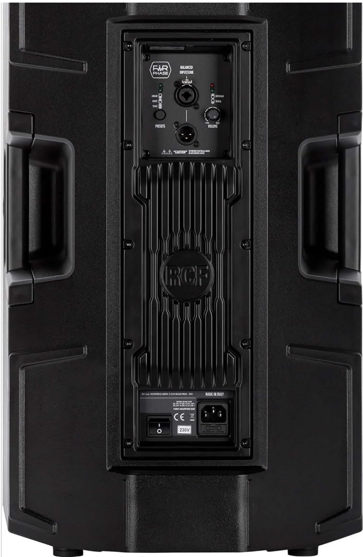
Figure 4.2: Rear panel of the RCF ART 915-A, displaying the balanced input/link, volume control, and preset buttons.
