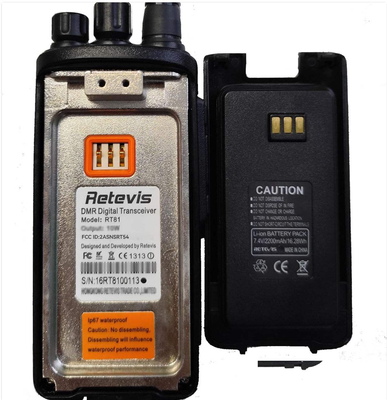
Image: Detailed view of the RT81 battery and its compartment, illustrating how to attach the battery.
