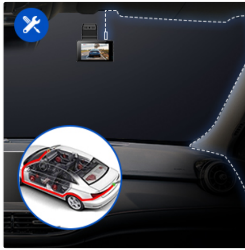
Image: A diagram illustrating the recommended cable routing for a neat and secure dash cam installation along the car's interior trim.
