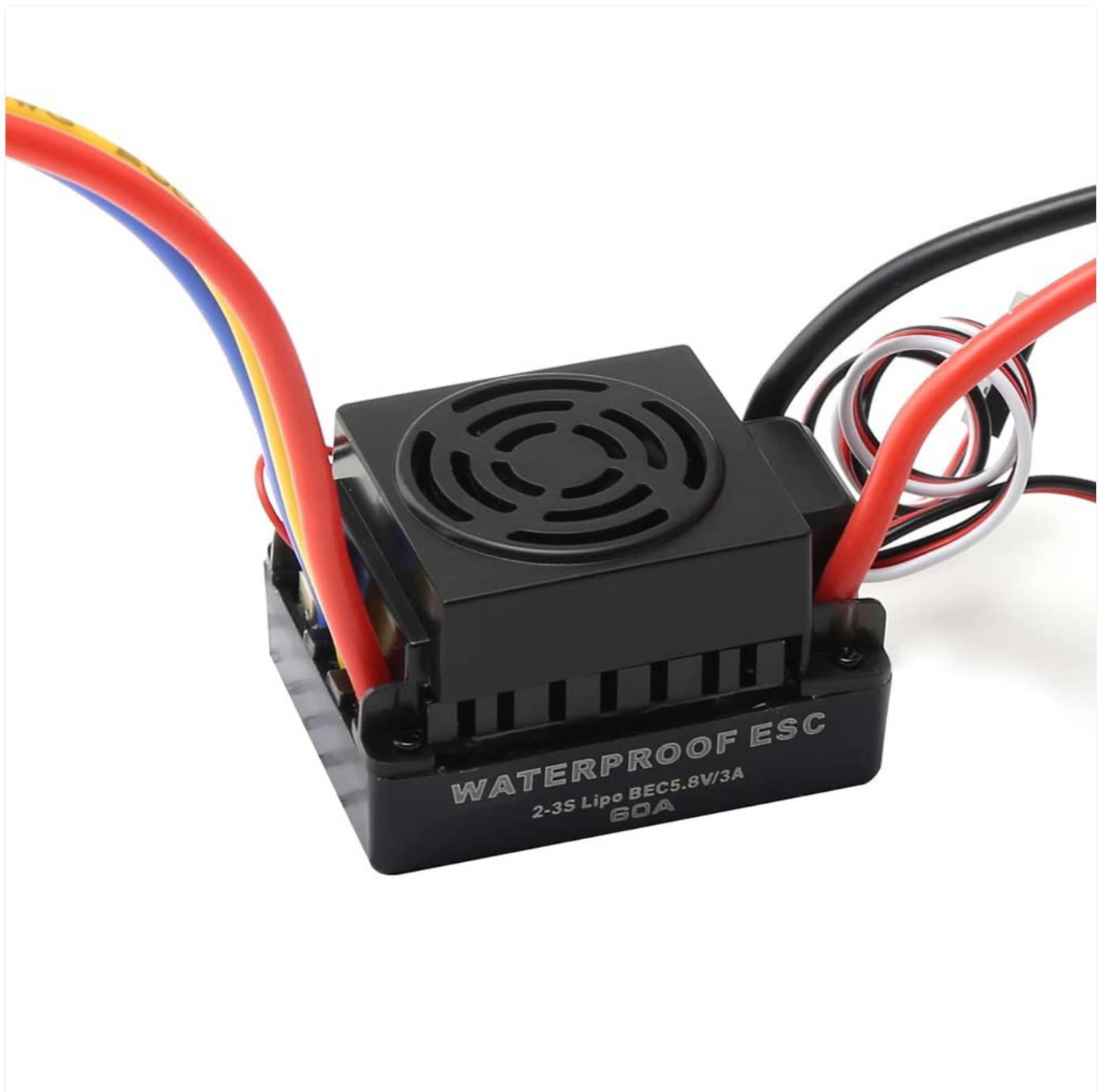
Figure 2: Close-up of the ESC showing the cooling fan and waterproof label.
