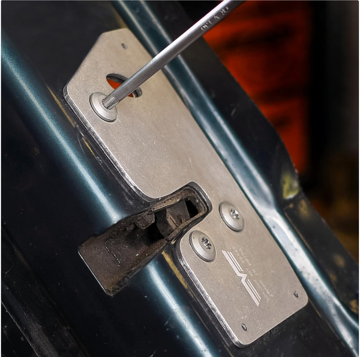
Figure 2: Illustrates the reinforcement plate being installed over the existing door panel, showing the alignment with the door latch mechanism.
