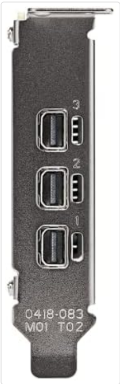
Image: A side view of the PNY NVIDIA T400 Graphics Card, clearly showing its three mini-DisplayPort outputs, which allow for multi-monitor setups.
