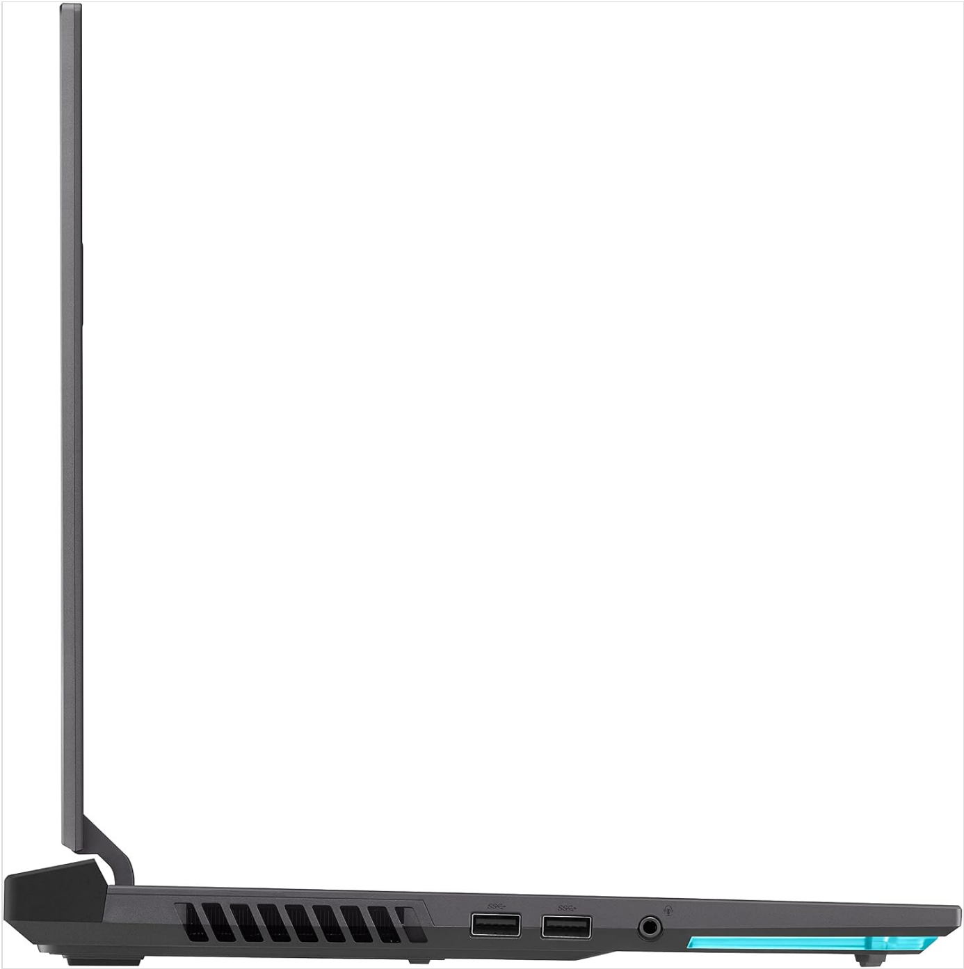
Right side of the laptop with USB Type-A ports and audio jack.
