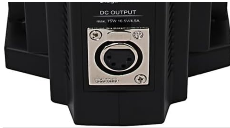
Figure 6.3: Front view of the charger with 4-pin XLR DC output.
