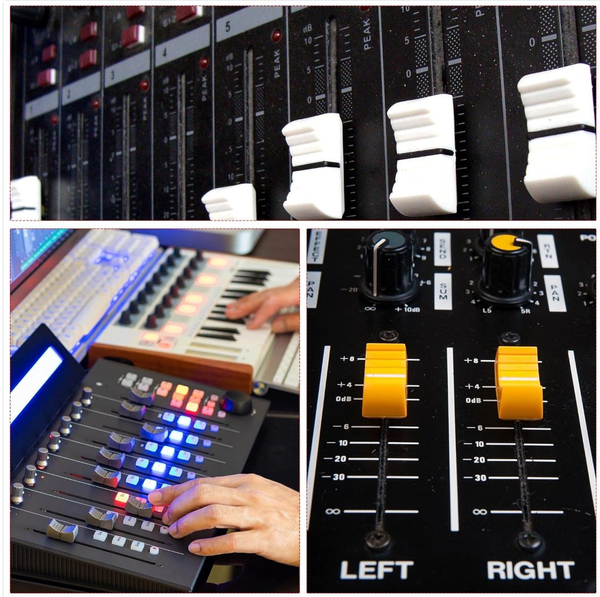
Figure 4.1: Examples of slide potentiometers integrated into audio mixing consoles, demonstrating their common application.
