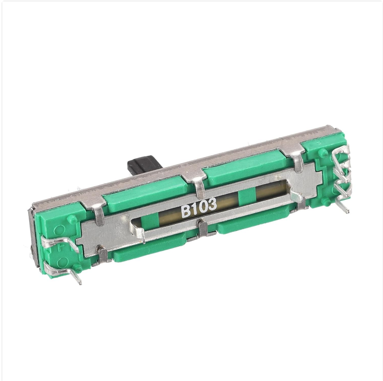
Figure 3.1: Underside view of the potentiometer, highlighting the terminal pins for soldering or connection.
