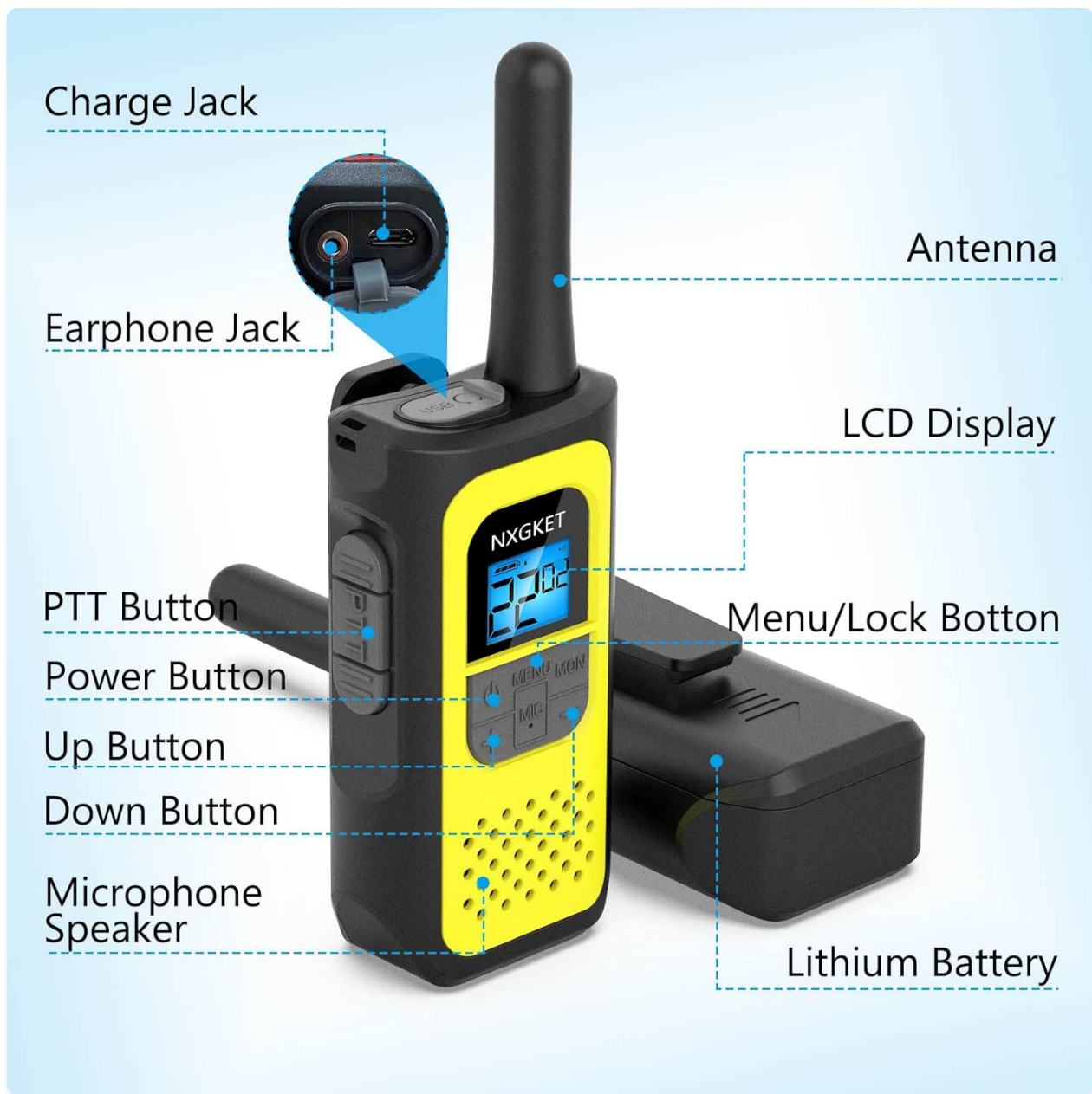
Figure 3: Labeled components of the walkie talkie.
