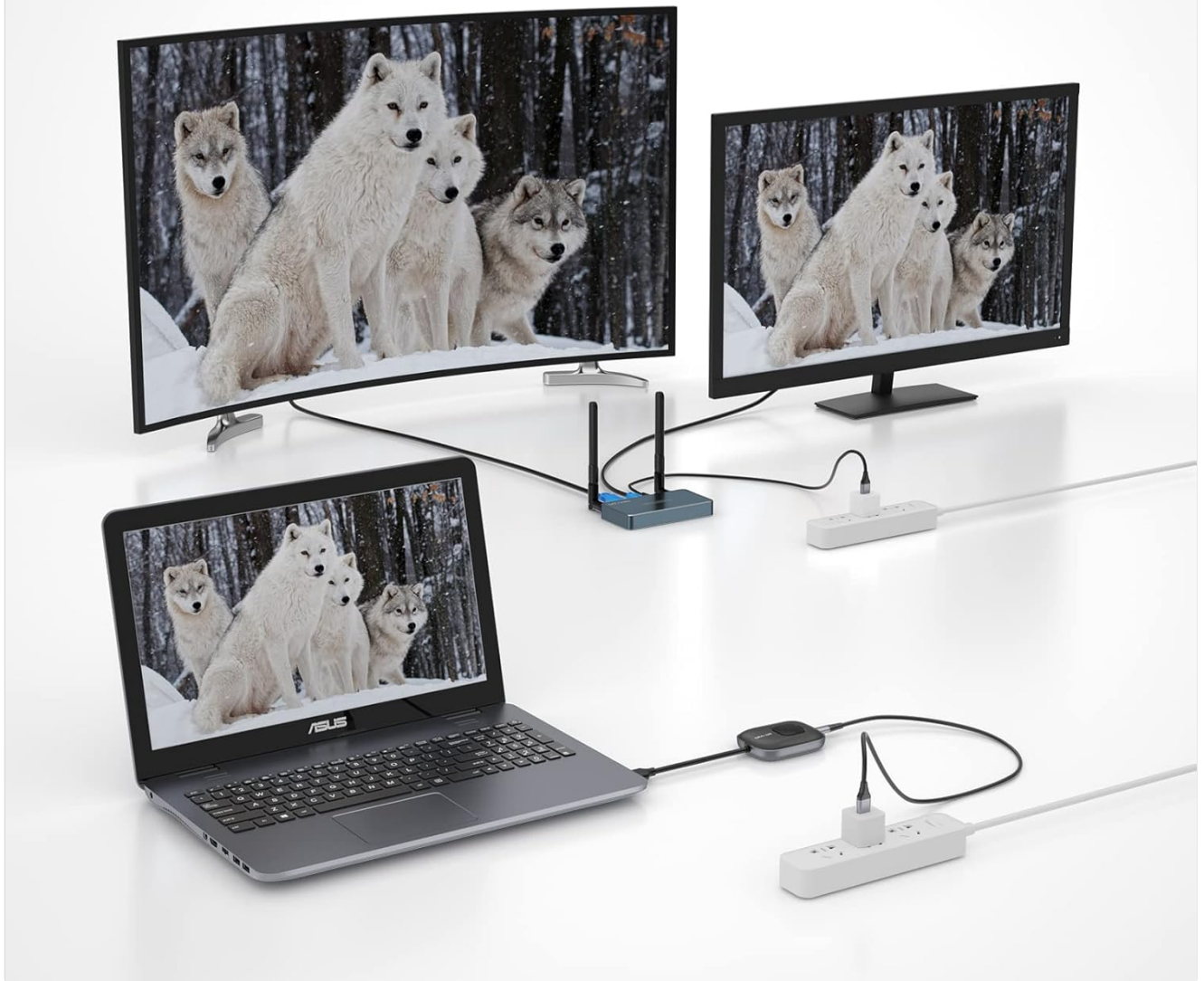
Image: A laptop connected to the MT-VIKI Wireless HDMI Extender, demonstrating its ability to output simultaneously to an HDMI television and a VGA monitor, displaying the same content on all three screens.
