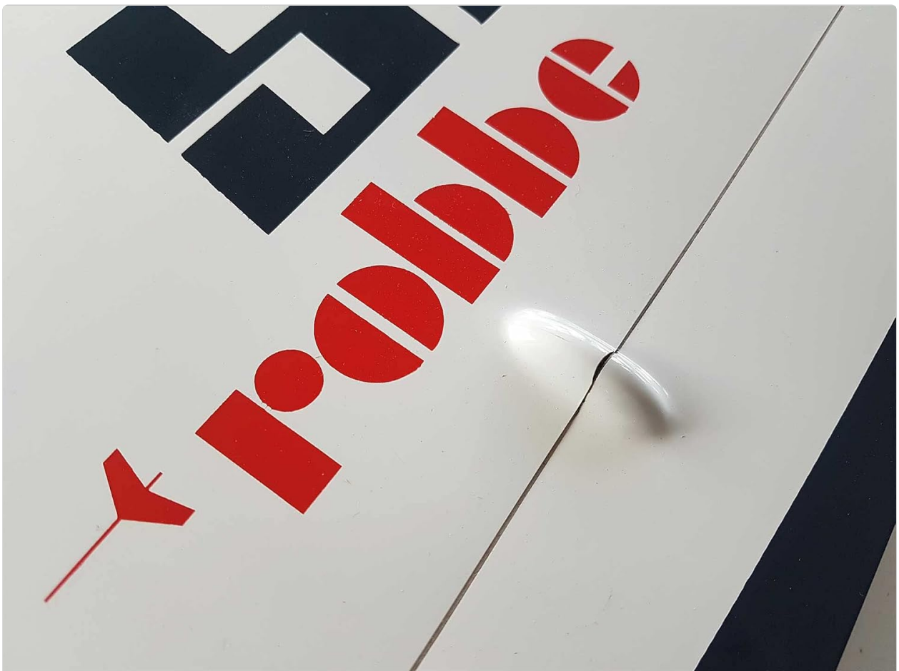
Figure 6: Close-up showing the continuous ailerons and flaps, which contribute to the model's high maneuverability.
