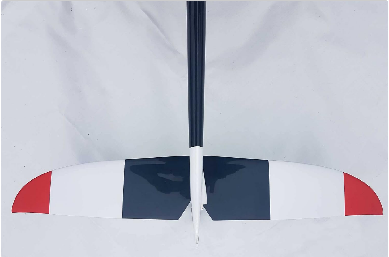
Figure 8: The tail section of the Scirocco S, showing the horizontal and vertical stabilizers.
