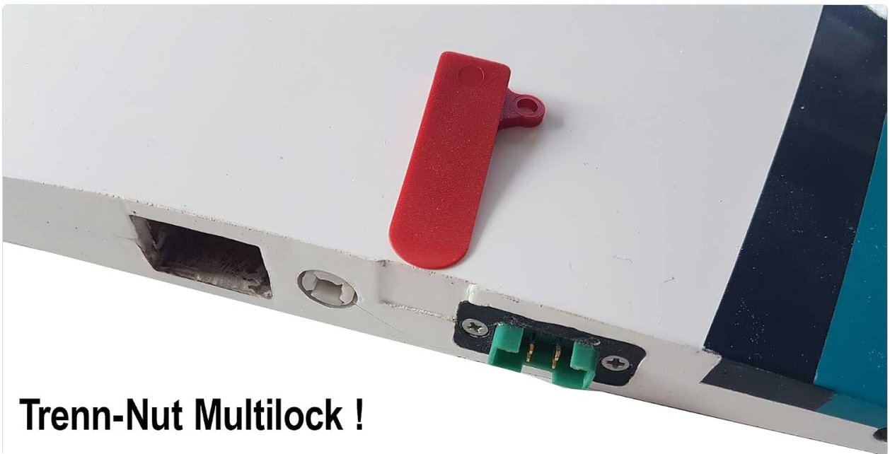
Figure 5: Detail of the Multilock separation groove, providing a secure and quick-release mechanism for wing attachment.
