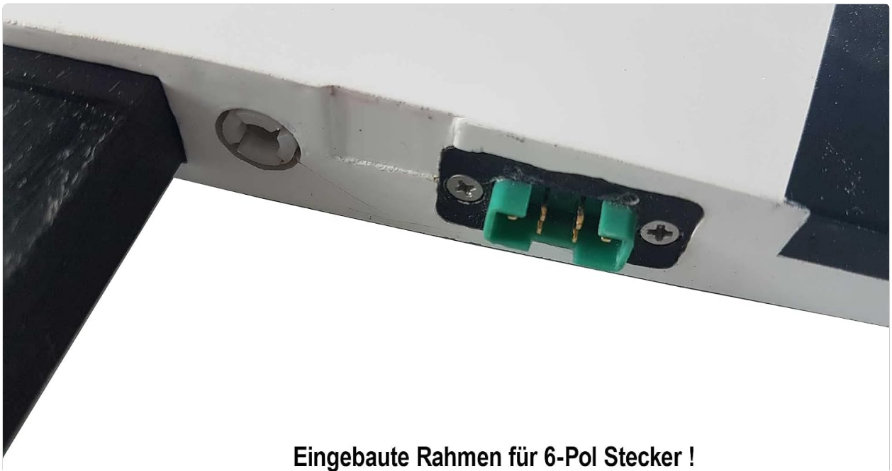
Figure 4: View of the built-in frames designed to accommodate 6-pole connectors, ensuring a clean and reliable electrical connection for the wing servos.
