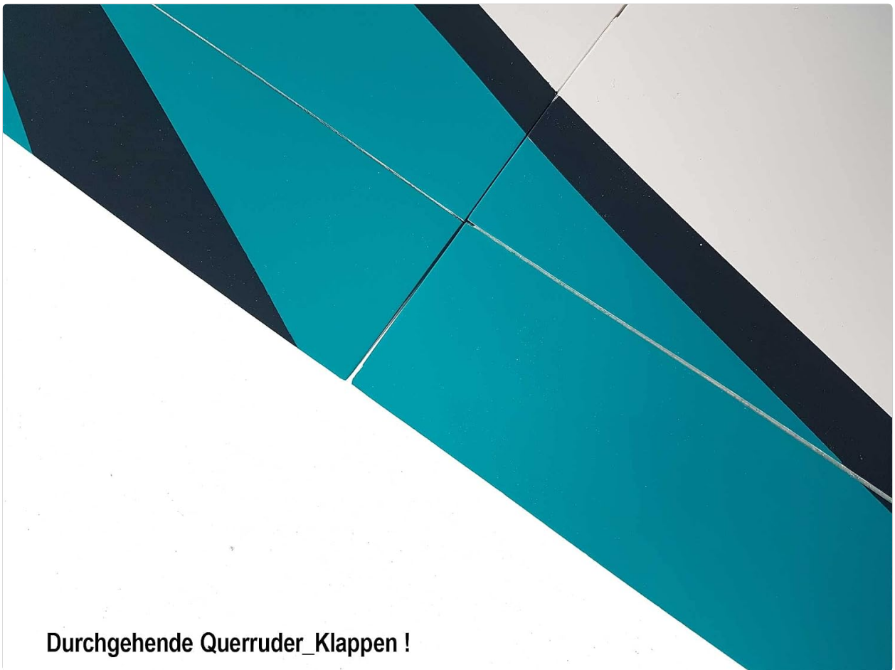
Figure 6: Close-up showing the continuous ailerons and flaps, which contribute to the model's high maneuverability.
