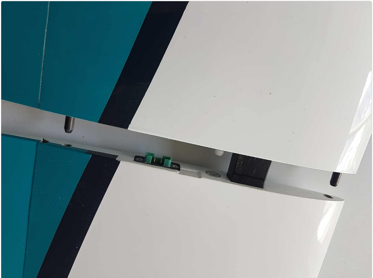
Figure 3: Close-up of the wing connection point, showing the green electrical connector for signal and power transfer.
