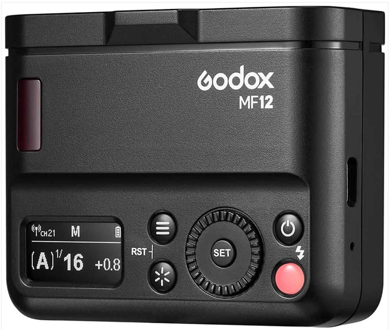
Image: A close-up view of the Godox MF12 flash control panel, showing the LCD screen, buttons for mode, reset, power, and the SET dial for adjustments.
